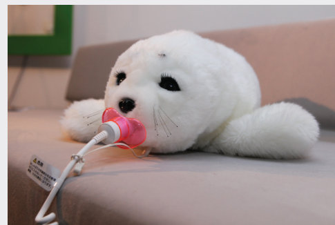
“Paro” by Japan's National Institute of Advanced Industrial Science and Technology (AIST) is an animal-like robot that has been in use in Japan and Europe since 2003 for therapeutic purposes—for example, providing care to people with Alzheimer's disease. Modeled on a baby seal, Paro registers environmental stimuli via two computers and five sensors that measure touch, light, sound, temperature and physical position. This enables it to interact with its human interlocutor. Paro is able to learn—it can recognize 50 different voices and responds to its name.” (Ars Electronica, “Paro,” 10 March 2011, https://www.flickr.com/photos/arselectronica/5514133373/ .)
